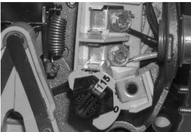
Figure 4: Motor Set for 115 Volt Operation
